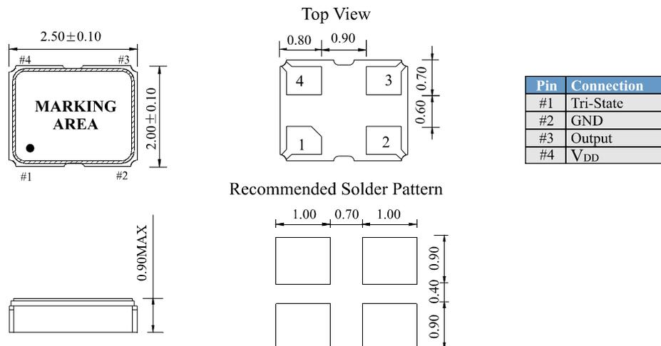
\*\*Note: 0.01uF bypass capacitor should be placed between V<sub>DD</sub>(Pin4) and GND(Pin2) to Minimize power supply line noise
